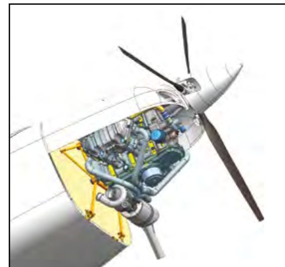
View of the installation of the CMD22 hybrid engine; image courtesy of CMD S.p.A.
